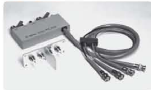
16048A/D/E BNC test leads Frequency: A: \leq 30 MHz, D: \leq 30 MHz, E: \leq 1 MHz Cable length: A: 0.94 m, D: 1.89 m, E: 3.8 m Maximum dc bias: \pm 40 V
