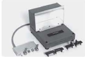
16065A axial and radial test fixture with safety cover Frequency: 50 Hz to 2 MHz Maximum externally supplied dc bias: \pm 200 V Blocking capacitor of 5.6 \mu F is connected in series with the Hc terminal
