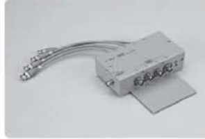
16065C external bias adapter Frequency: 50 Hz to 1 MHz Maximum externally supplied dc bias: \pm 40 V Blocking capacitor of 50 \mu F is connected in series with the Hc terminal
