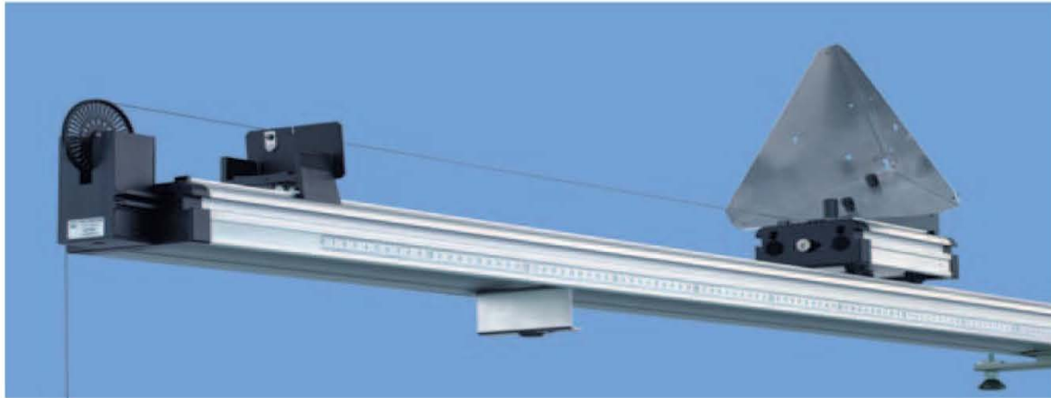
Experiment setup on a Doppler radar with track and trolley. The trolley is accelerated to typical laboratory speeds by means of a traction weight.
