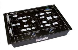
Both the phase and amplitude can simultaneously be varied in Quadrature Amplitude Modulation (QAM). More bits can be send in each symbol, but an unavoidable decrease in the tolerance for noise results. Thus, 16-QAM with many possible values works very well in wired & wireless channels.
