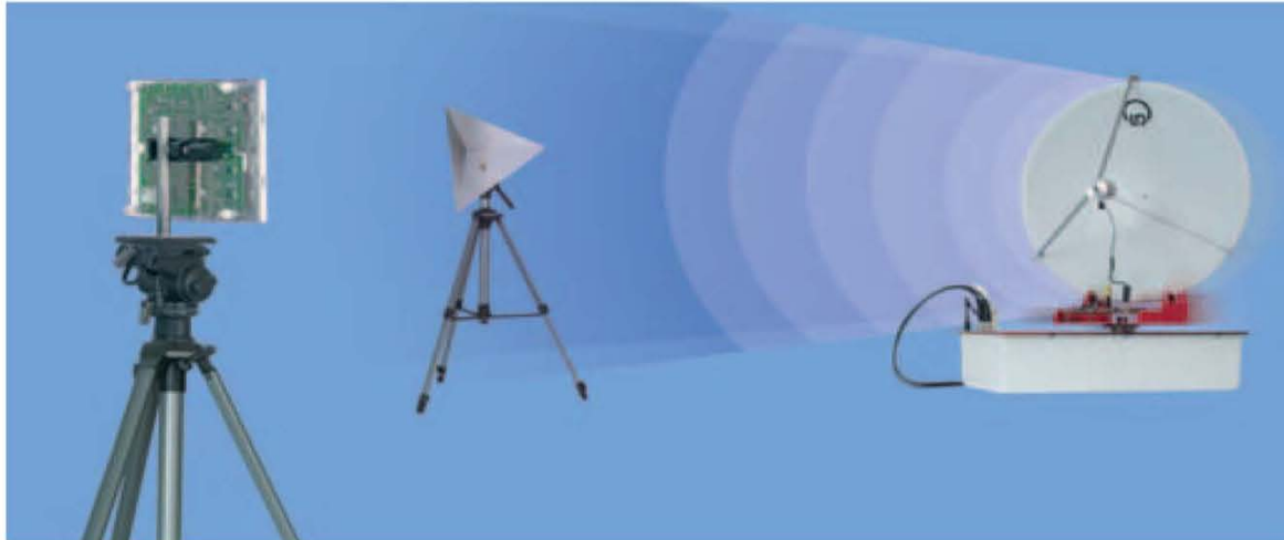
Experiment setup for ultrasonic radar with corner reflector and transponder
