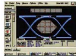
Eye diagram analysis. Take advantage of the easiest and most intuitive method for viewing high-speed digital communications waveforms.
